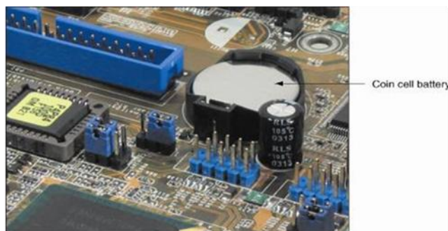
Figure 5-24 The coin cell is the most common type of CMOS battery
