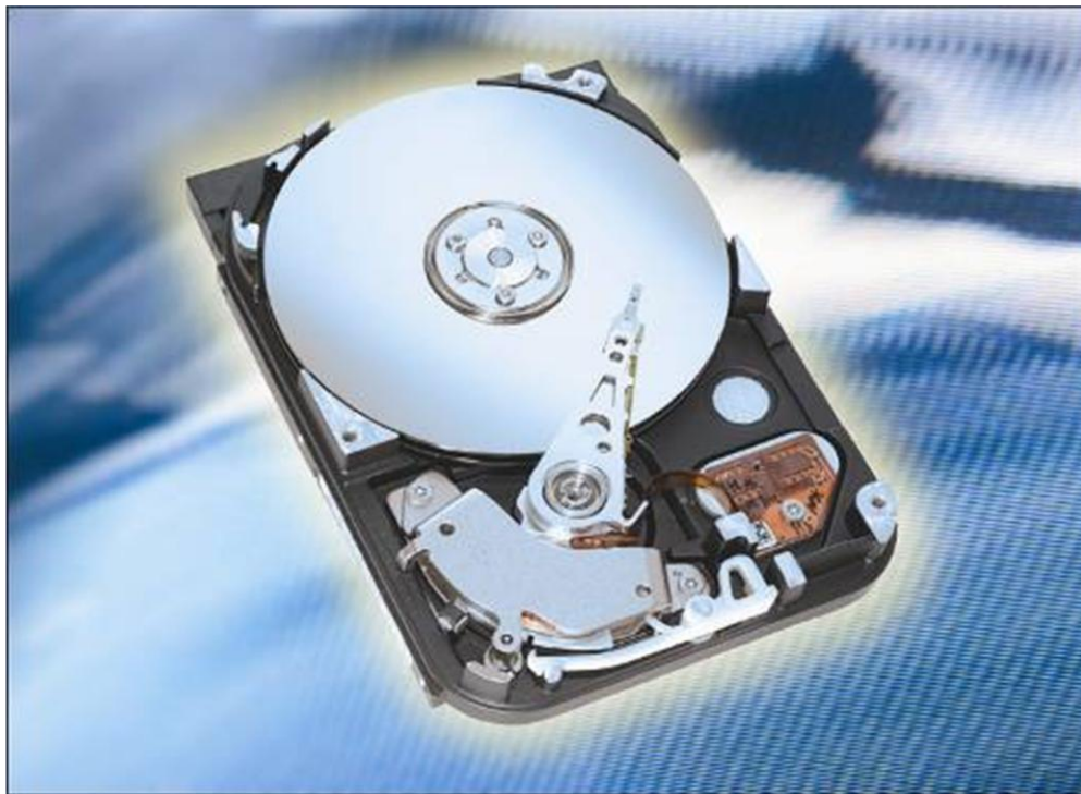
Figure 1-16 Hard drive with sealed cover removed
