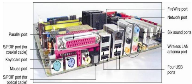
Figure 1-9 All hardware components are either located on the motherboard or directly or indirectly connected to it because they must all communicate with the CPU
