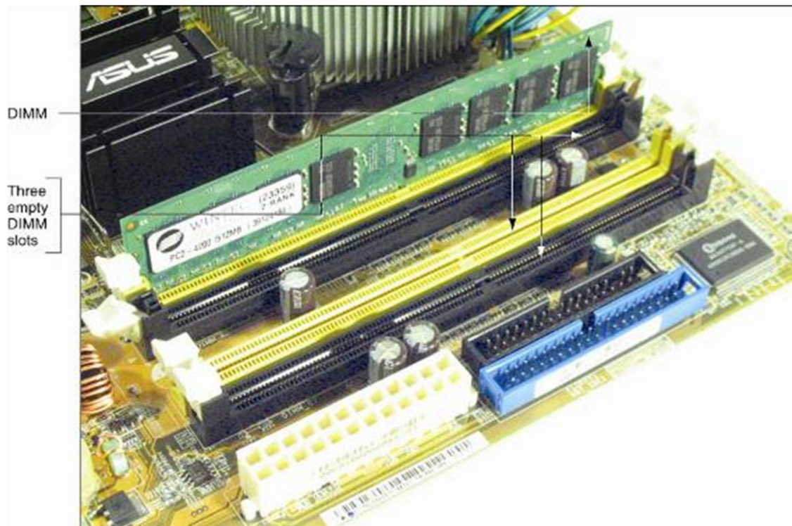
Figure 1-14 A SIMM, DIMM, or RIMM holds RAM and is mounted directly on a motherboard
