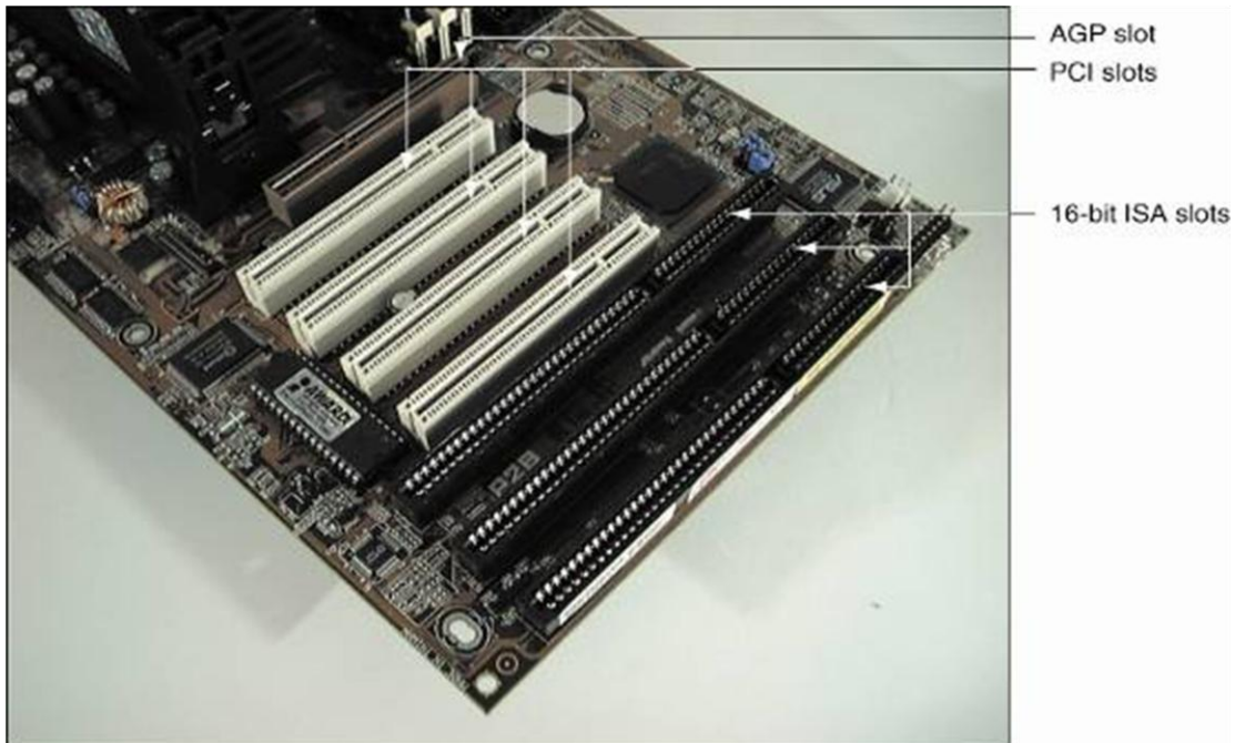
Figure 1-29 PCI bus expansion slots are shorter than ISA slots and offset farther; the one AGP slot is set farther from the edge of the board
