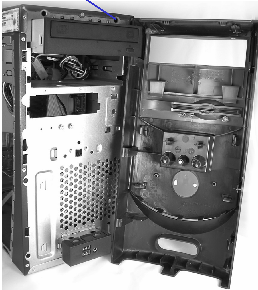
Exhibit 3-5: Front-cover alignment and catch mechanisms
