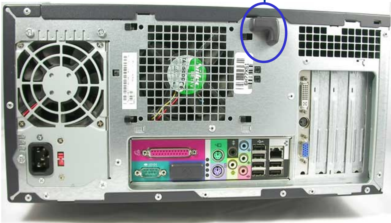
Exhibit 3-3: Typical slide latch used to secure a case
